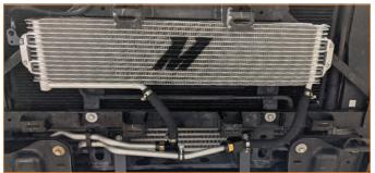
**15.** The 2017–2019 grille will not clear the driver-side rubber transmission cooler line. A portion of the lower grille will need to be trimmed.
