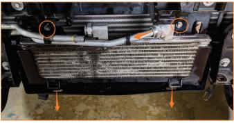
**11.** Install Mishimoto Transmission cooler to the front of core support using supplied brackets. To ease installation, all brackets should be installed, and core centered in position before hold-down bolts are tightened, be sure to tighten brackets evenly (4x 4mm hex socket).
