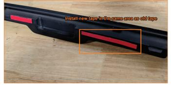
**17.** In order to re-install rain guard from step 1. Old double-sided "emblem tape" will need to be removed and new tape applied.
