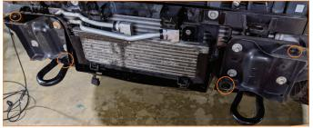
**08.** Unclip plastic transmission cooler line brace, as well as removing plastic trans cooler line quick disconnect covers.
