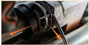
**10.** Unbolt stock transmission cooler and un-clip lower shield by pulling down on the shield. Remove longer transmission cooler line at the same time as the stock transmission cooler if more clearance is needed (2x 10mm bolts).
