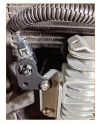
13. Install mounting brackets using stock transmission cooler mounting bolt locations and hardware, clip lower shield to brackets with supplied tree clips. Install P-clip around transmission line as shown. Refer to product product diagram for bracket assembly.
