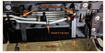
**14.** Install rubber lines with supplied worm gear clamps. The longer line gets installed on the driver's side of the cooler.
