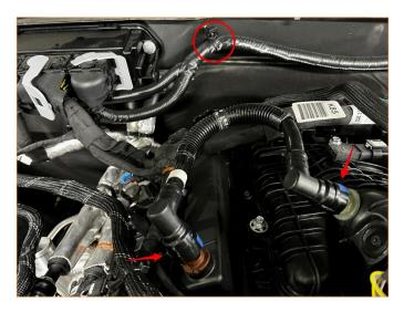
02. Remove the nut and the plastic cap, exposing the two M6 studs for mounting the catch can bracket.
