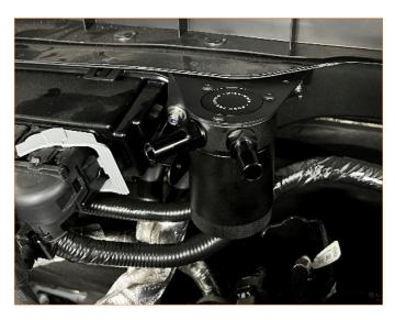
**04.** Attach catch can hoses as shown and secure with provided worm gear clamps.
