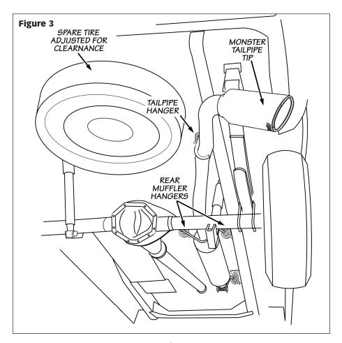
**10.** With the exhaust positioned properly, begin to tighten the clamps starting with the ones closest to the front of the vehicle and working your way back. Torque the exhaust clamps evenly to 35 ft-lbs. Make sure that each slip is fully inserted  $(+/- \frac{1}{4}'')$ .
