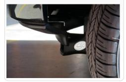
19. Check to make sure the Scoop assembly does not interfere with the wheel or wheel well liner. Turn the wheel in both directions while trying to simulate full
