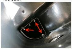
11. Locate these two bolts from behind the front bumper. Using a 10mm socket, remove the two bolts.
