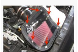
3. Loosen both hose clamps on the hump adapter and the slide the hump adapter over the intake tube. Then remove the Adapter tube and Air Filter from the air box.
