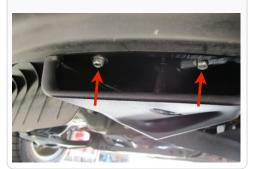
15. Double check to make sure all hardware on the scoop is securely fastened and all parts are properly positioned.
