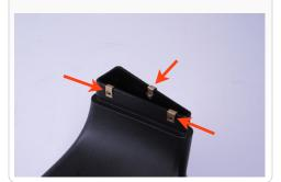
6. Slide the Scoop Channel (C) over the Scoop Base (D) and attach using the three supplied #10-32 Screws (B) and Sealing Washers (A).
