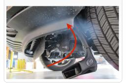
$9. \ \ \, \text{From inside the air box grab the top of the}$ Scoop assembly and align with the three holes in the air box. Note: It be necessary to move some wiring harnesses out of the way to gain clearance for the scoop assembly.
