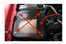
18. Reposition the intake tube and reattach the hump coupler to the filter adapter tube. Tighten all hose clamps when you are satisfied with the position.
