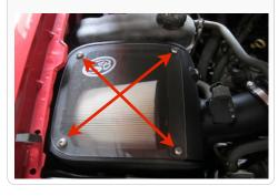
5. Carefully remove the Air Filter/ Adapter tube assembly up out of the air box.
