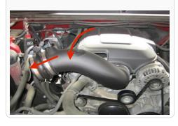
19. Reconnect the MAF sensor wiring harness (and Pressure Sensor if equipped).
