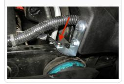
15. Reattach the fender liner to scoop using two 1/4"-20x1/2" Hex Screws (D) and 1/4" Washers (E). Chevy models will use one 1/4-20x1.0" Hex Screw (C) securing the fender liner to the Chevy Bracket (G).
