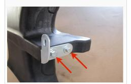
11. Chevy Models Only! Attach the Chevy Bracket (G) to the Scoop (A) using two 1/4"-20x1/2" Hex Screws (D) and 1/4" Washers (E). Then install the Clip Nut (B) onto the bracket
