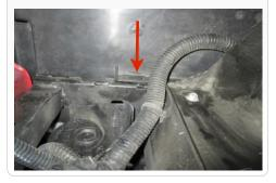
8. Using a 7mm socket and extension, position the ratchet through the air box and go around the support to access the other screw mounting the plate. This screw will be reused with the new scoop. Remove the plate from the vehicle from under the truck by pulling down and towards the motor.
