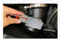
3. Loosen the two hose clamps on the Hump Coupler and one on the throttle body. Then rotate the assembly out of the way.
