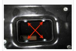
14. Attach the Mounting Bracket to the front support using the OE screw and a supplied 1/4" Washer (E).
