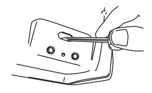
Install Brackets onto vehicle. On Passenger side install Rear Rail Mounting Bracket (35) and Front Linkage Mounting Bracket (33) using the Hardware provided. 4 Conical washer bolts (9), 4 Button Head Torx (19), washers (20) and Flange Nuts (17). Once bolts are tightened up to vehicle torque Conical washer bolts (9) to 16 ft-lbs and Button head Torx to 6ft-lbs.
