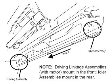
Set Reinforcement Plate in place and locate with rivet nuts. Drill hole using an 1/8" drill bit. After drilling apply paint to prevent rusting
