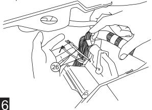
Insert controller (7)into tie-wrap (25) loops and cinch down securely. The tie-wraps should cinch down into channels on controller surface.
