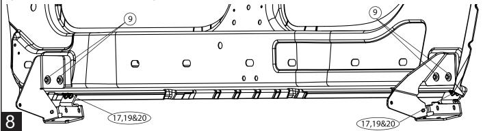
Insert and position 6 Carriage bolts (16) into slot on rail (4). Insert from either end of rail. Using Flange Nuts (10) provided assemble rail to Brackets using the 2 outer bolts on each side. Next install Flange Bolt (14) and Flange Nut (10) onto bracket tab. Torque flange nuts to 16ft-lbs. Install Light Bracket (29) using Flange Nut (10), leave loose to allow for adjustment. Driver side shown. Dimensions shown are for reference.
