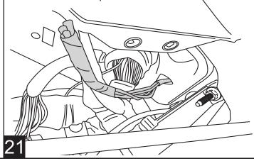
Route the two Wire Harness (6) legs down over the wheel wells toward Motor Linkages, long leg across to the passenger side. Secure harness with tie wraps (24).
