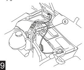
Locate large rubber wire boot on driver side firewall as shown below. Slice small opening as shown below to run trigger wires through.
