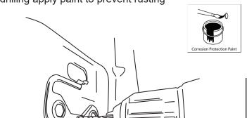
Once hole is drilled insert a piece of string or wire through hole in Reinforcement Plate. Set plate into position.
