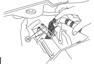
Insert controller (7) into tie-wrap loops and cinch down securely. The tie-wraps (25) should cinch down into channels on controller surface.
