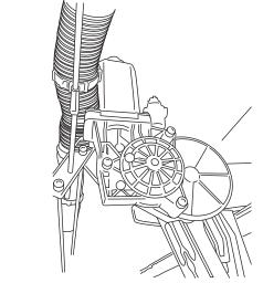
Affix LED lamp (#26) to Light bracket (#29) on rail. Slide bracket into desired position and tighten using 5/32" Allen key.
