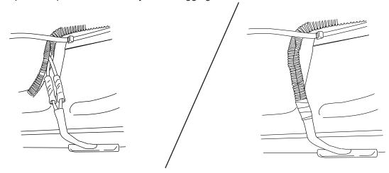
**OBD II install:** Use Supplied Posi Twist connectors to attach the Plug and Play Module to the Harness. Attach matching colors on the harness to the wires on the module. Plug in module to OBD II port on the vehicle. Secure harness with supplied tie wraps.
