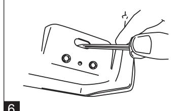
Install Brackets onto vehicle. On Passenger side install Rear Rail Mounting Bracket (37) and Front Linkage Mounting Bracket (35) using the Hardware provided. 4 Conical washer bolts (9), 4 Button Head Torx (19), washers (20) and Flange Nuts (17). Once bolts are tightened up to vehicle torque Conical washer bolts (9) to 16 ft-lbs and Button head Torx to 6ft-lbs.
