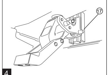
Locate Rear most set of threaded holes on the frame just forward of rear suspension. Vehicle shown has Vehicle Stability Control lines. Tighten screws to 16 ft-lbs.
