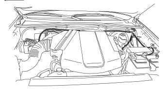
Note: Run loom with Green/Yellow and Pink/Black Trigger wires down drivers side of vehicle.
