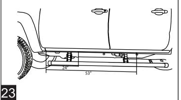
Drill a 9/32" hole through the pinch weld at marked locations. Debur all holes.
