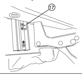
Snug bolts to allow for adjustment at a later step.
