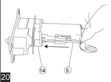
Slide rubber grommet on Wire Harness into slot of Motor Cover. Slide Motor Cover over Motor.
