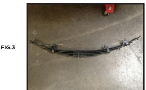
**11**. Put the bottom half of the pack back in the vehicle guiding the center pins up through the upper 3 leaves. A long drift punch helps to align the holes. It may be helpful to loosen the 2 C-clamps slightly on the front and rear to help shift all leaves into position. Use a large C-clamp near the middle to pull everything together until you can get the nuts started on the center pin.
