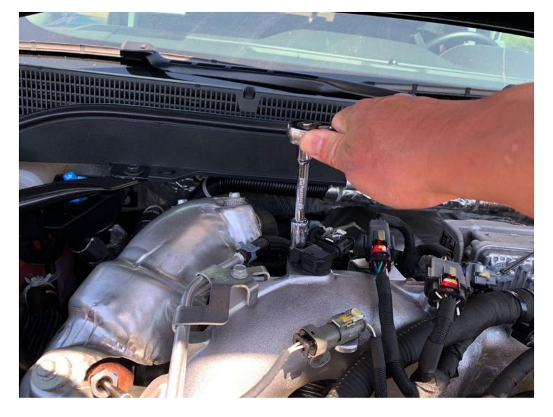
Remove the M6 Hex Head Flange Screw and keep it to use in Step 4. Do not disconnect the harness from the MAP Sensor.
