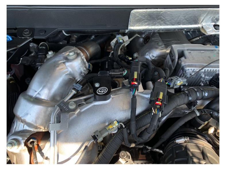
Finished installation should look like this as shown. Make sure the MAP Sensor and Harness are free from rubbing other components that may cause any wear or damage.
