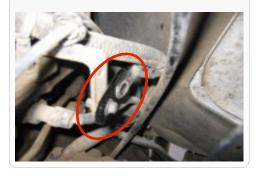
15. Place the M6 Bolt (P) through the dip stick tube bracket and the S&B Dip Stick Bracket (O) and thread the M6 Lock Nut (Q) on the bolt, leave loose until the upper mount is in place.
