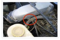
5. Remove the 4 bolts that secure the elbow to the manifold and remove the elbow from the vehicle. Careful not to let any debris fall into the manifold. Note: If the OE bolt threads were corroded and rust deposits have fallen through the bolt holes into the manifold use a vacuum to clean it out
