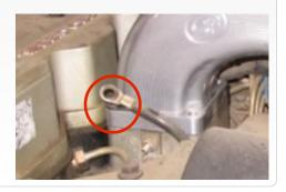
18. Place a M8 Washer (D) over each stud and thread on the M8 Lock Nuts (C). Torque both the lock nuts and the screws to 145 ln. lbs. If you use a crow foot to torque the nuts, see the crow foot calculation on page 3. Maintenance Note! Check and retorque the M8 Lock Nuts (C) 100 miles after initial installation. Periodically checking and retorquing the locks nuts is also good practice as they loosen over time due to engine vibrations.
