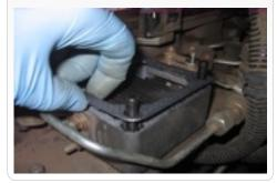
14. Remove the bolt at the lower dip stick tube bracket. Place the S&B Dip Stick Bracket (O) (oval hole) in its place and secure loosely with the OE bolt.
