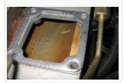
8. This kit has 2 Long Studs (J) and 2 Short Studs (H), to determine the correct stud length for your truck, thread each a long and short stud (short threaded end first) into the manifold bolt holes farthest from the valve cover. Measure the height of the stud from the heater grid block upward. Use the studs that are approximately 1.125" tall. (See pg. 5 for details)
