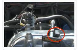
4. Pull the prong out that secures the wiring harness to the elbow and push the harness back away from the elbow.
