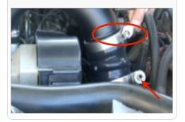
20. Secure the dip stick tube upper bracket to the Elbow. Apply thread locker to the 5/16" x 1/2" Hex Bolt (B). Then place the Flat Washer (A) on the 5/16" x 1/2" Hex Bolt (B). Place the bolt and washer through the upper bracket and place the Rubber Washer (M) and the other Flat Washer (A) under the bracket and thread the bolt into the elbow and secure. Do not exceed 30 In. lbs. Then tighten the two bolts at the lower bracket.
