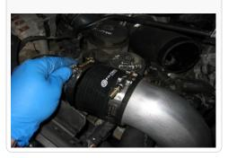
17. Position the upper T-bolt clamps as to not hit the hood when closed and torque them both to 50 ln.lbs.
