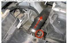
**6.** Remove the 4 bolts that secure the OE elbow to the intake manifold and remove the elbow from the vehicle. Be careful not to let debris fall into the intake manifold. *Note the longer bolt's location*.
