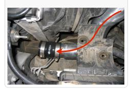
15. Insert the S&B Elbow (A) into the Straight Coupler (F) and align the bolt holes with the intake manifold. Be sure the OE Oring is still in place and clean both mating surfaces prior to installing.
