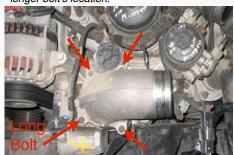
7. Apply sealant (Teflon tape) to each 1/8"NPT Plug (E) and insert the plugs into the ports you will not use on the elbow. Use 3/16" Hex drive and torque the plugs to 40 In.lbs.
