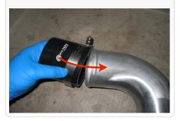
14. Place the other supplied T-bolt Clamp (G) over the end of the Straight Coupler (F).
