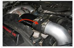
**18.** Reinstall the Intake or OE air cleaner and filter removed in Step 3.
