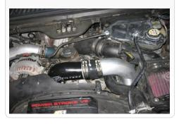
11. Place one the supplied T-bolt Clamp (G) over the Straight Coupler (F) and slide it on the upper end (Large diameter) of the Boost Tube (H).
