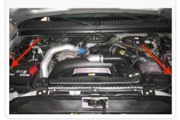
2. Optional step, to allow better access to the elbow. Use a small flat head screwdriver and pry the clips open and pull up working your way across to remove the upper fan shroud.
