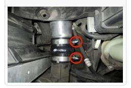
16. Insert the M6x30mm Bolts (D) and M6x93mm Bolts (C) in the proper locations and torque to 100 ln.lbs.
