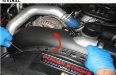
3. Remove the OE (or aftermarket) intake to gain access to the clamps of the OE boost tube. Follow the manufacture's procedures for removing the intake.
