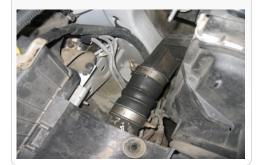
4. Loosen the hose clamp at the OE elbow and pull the adapter off the elbow.
