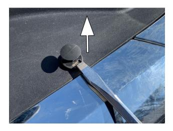
Lift-up the factory air scoop cover and remove it from the vehicle. Set it to the side, to be re-installed later
