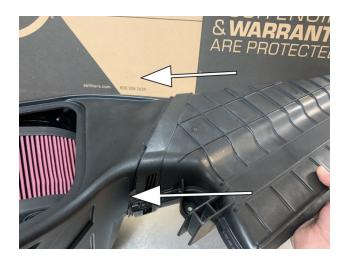
Drop the Complete S&B Cold Air Intake assembly and factory scoop into the vehicle. Lining up grommets, Push in firmly onto the vehicles factory mounting locations
