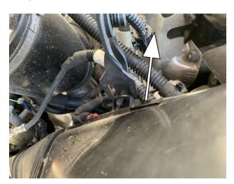
Using a 5/16" driver or socket, loosen the hose clamp on the factory tube connected at the turbo inlet. Access can be a challenge. If necessary use a socket extension to access the worm drive of the hose clamp
