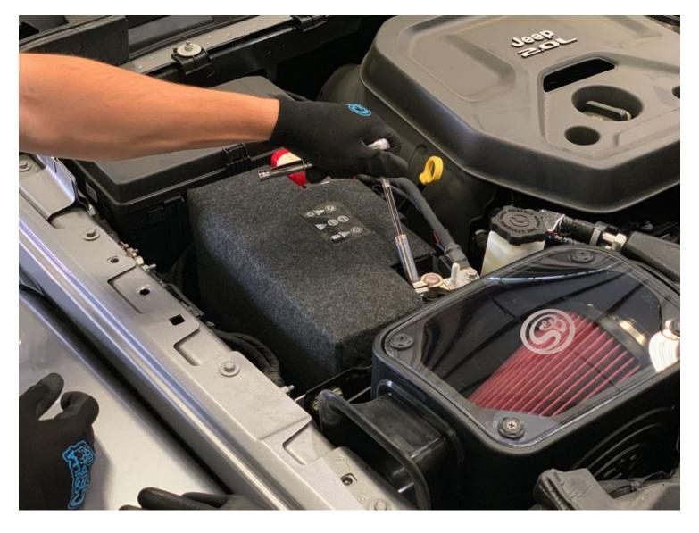
Reconnect the negative terminal on battery. Inspect your installation, make sure the kit is properly positioned and all fasteners are secured. S&B Filters recommends keeping all stock parts in case you would ever need to reinstall the stock intake.
