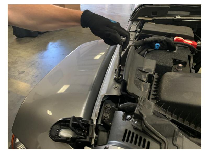
Remove the bolt securing the stock intake box to the fender.
