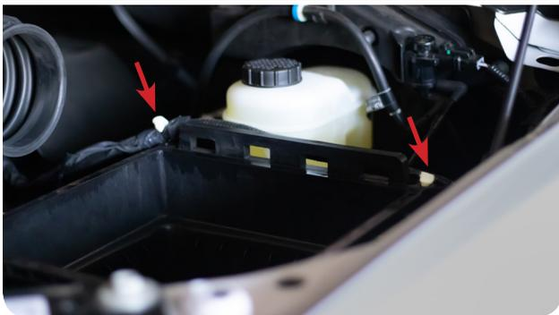
**10** Remove the plastic rivets on the stock air scoop using a flat head screwdriver. First pop the center up to unlock the rivet, then remove the complete rivet.
