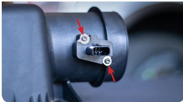
**21** Install the MAF sensor onto the Large Intake Tube (B), using the provided MAF Mount (R), MAF Gasket (S), and Screws (T).
