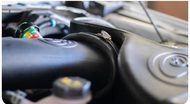
**31** Slide the Air Filter over the Large Intake Tube until the tube bottoms out on the step on the inside of the filter flange, then tighten the Hose Clamp.
