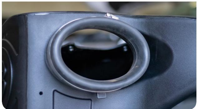
**19** Install the Front Inlet (I) onto the S&B Air Box. Use 2 of the supplied Plastic Rivets (J) on each hole, pinching them together tightly to lock them in place.
