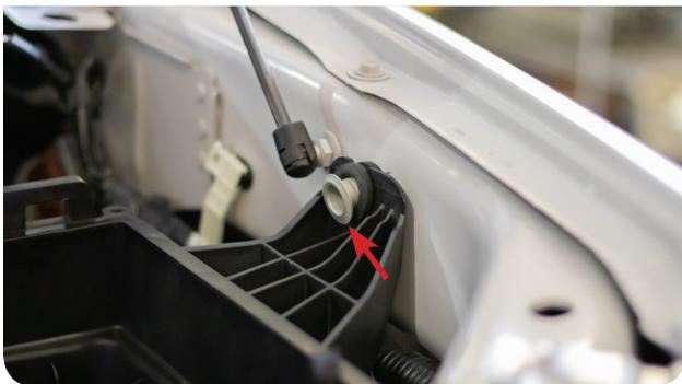
**8** Remove the grommet from the stock air box by pulling up. Set the grommet aside, it will be reused in Step 16.
