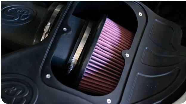
**32** Install the larger end of the Small Intake Tube (C) into the Coupler on the Large Intake Tube.
