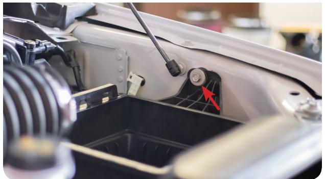
**7** Remove the metal bushing from the stock air box pulling it from the inside. Set the metal bushing aside, it will be reused in Step 17.
