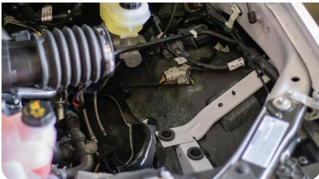
**12** Completely loosen the hose clamp connecting the stock intake tube to the turbo inlet tube.
