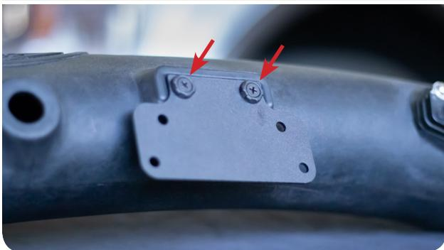
**24** Install the Push In Cable Ties (V) into the 4 holes in the bracket.
