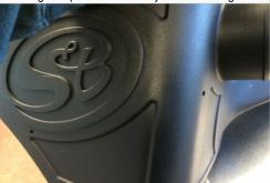
26. Secure the Front Inlet (G). Firmly push down on the center pin of the Plastic Rivet (I) until it locks into the closed position.
