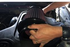
21. Feed the Air Intake Tube (B) underneath the coolant line through the Rubber Cuff (C) until the bead on the air intake tube meets up to the rubber cuff. Slide the Air Filter (D) over the tube until the tube bottoms out on the filter flange step.
