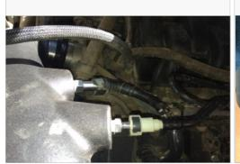
25. Insert the two wire clips disconnected in Step 7b into the holes on the side of the Air Box (A). Use zip ties to secure any loose wires or harnesses away from any hot surfaces and/or moving components that may cause damage.
