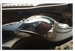
30. Reconnect the negative terminal on the battery. Inspect your installation, make sure the kit is properly positioned and all fasteners are secure. Affix the ID/CARB label near the kit under the hood. The installation is now complete.
