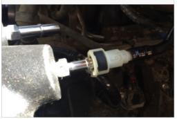
24b. Reconnect the PCV hose. Push in the connector over the Quick Connect Fitting (Q) until you hear it snap into place.
