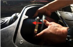
22. Tighten the Hose Clamp #88 (J) at the Air Filter (D).
