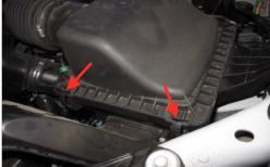
4. Lift and remove both the lid and air filter.
