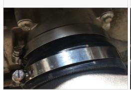
20. Place the Air Filter (D) and Hose Clamp #88 (J) inside the Air Box (A). Turn the filter sideways and slide it into the air box.
