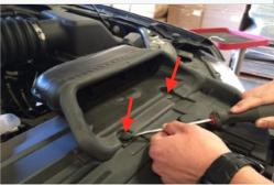
**13.** Remove the grommet and metal bushing from the stock air box. Removing the metal bushing first will make removing the grommet easier.
