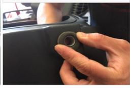
17. Install the Front Inlet (G). Use the supplied Plastic Rivet (H) to secure the front inlet to the Air Box (A). Use two plastic rivets on each hole and pinch them together to lock them in place.
