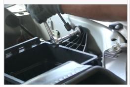
12. Lift and remove the stock air box.
