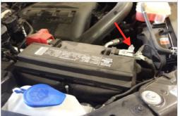
4. Loosen the hose clamp at the tube leading 5. the turbo inlet on the driver side.
