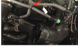
21. Install the Air Box (A). Make sure that the box prongs are aligned with the factory grommets. Push down on the air box to make sure that the prongs are completely seated.
