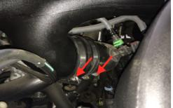
33a. For 2015-2016 Models and 2017 2.7L EcoBoost Only. Insert the two wire harness clips disconnected in Step 11 into the holes on the side of the Air Box (A). For 2017 3.5L EcoBoost Only. Insert one wire harness clip into the hole under the S&B Logo and use zip ties secure the other wire harness clip away from any hot surfaces and moving components that may cause damage.
