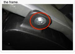
16. Install the 1/4-20 Screws (V), Split Lock Washers (U) and 1/4" Flat Washers (W) to secure the Snorkel Tube (S) onto the Air Box (M).
