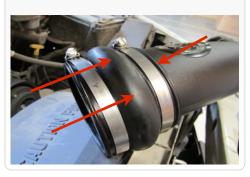
24. Slide the Step Coupler (B) with #56 #60 Hose Clamps (A & C) onto the throttle body. Tighten only the #56 Hose Clamp.
