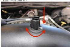
23. Install the Hump Coupler (G) with two #72 Hose Clamps (F) onto the Intake Tube (E). Stop when the coupler reaches the stop bead.
