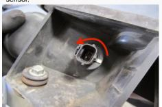
22. Insert the supplied Grommet (D) into the Intake Tube (E) and carefully push the temperature sensor into Intake Tube (E) using a twisting motion. Be sure to match the
