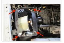
Note the stock temperature sensor orientation then carefully turn it counter clockwise and pull it out of the stock resonator. Remove the O-ring from the
