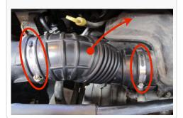
**3.** Loosen the two screws on the resonator assembly using a 10mm socket. Disconnect the temperature sensor wiring harness from the sensor.
