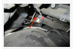
**9.** Using a 13mm socket, remove the other 2 screws securing the intake box tray inside the wheel well.
