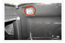
15. Secure the bottom of the Air Box (M) From inside the wheel well, install the M8 Screw (K) and Flat Washer (L). Then fully tighten both screws mounting the air box to
