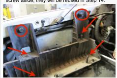
7. Remove the screws securing the wheel liner using a 8mm Wrench/Socket.
