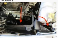
14. Use the stock screw removed in Step 6 to secure the Air Box (M) to the frame. Leave the screw loose.
