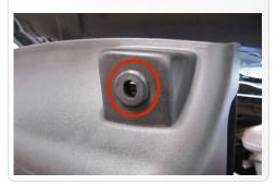
11. Determine if you want to install the Snorkel Plug (T) onto the Snorkel Tube (S) or leave it open. See the "Air Box Plug Testing" note on Page 3 for more information. If the Box Plug is desired, install 1/4-20 Screws (V), Split Lock Washers (U) and 1/4" Flat Washers (W).
