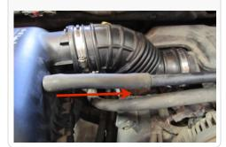
6. Carefully lift the stock intake box out of the four pins from the intake box tray. Remove the two screws securing the intake box tray to the frame using a 13mm socket. Set one screw aside, they will be reused in Step 14.
