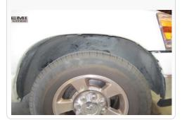
8. From inside the engine compartment, carefully pull the wiring harness clip out of the wheel liner. Then set the wheel liner aside.
