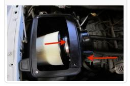
19. 2003 Models Only: Install the Breather Hose (Z) onto the oil fill reservoir and stem on the Adapter Tube (H) with the #8 Hose Clamps (Y). Tighten the hose clamp and secure using the supplied Cable Tie (Y).
