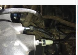
25. Insert the two wire clips disconnected in Step 7b into the holes on the side of the Air Box (A). Use zip ties to secure any loose wires or harnesses away from any hot surfaces and/or
