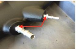
17. Install the Air Box (A). Make sure that the box prongs are aligned with the factory grommets. Push down on the air box to make sure that the prongs are completely seated.
