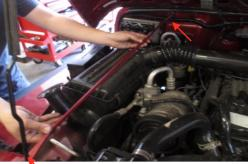
6. Lift up and pull the stock intake out. It should come out as one piece.
