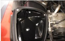
14. Insert the Air Filter (B) into the Air Box (A). Make sure the hose clamp is accessible. Push the connected Air Tube (F&H) through the Rubber Cuff (E) until you can slip on the air filter. Tighten the #88 Hose Clamp (L) at the air filter to secure the air filter to the tube.
