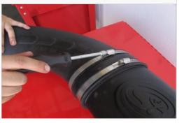
11. Install the Rubber Cuff (E) with the #104 Hose Clamp (M) on the Air Box (A). Tighten the hose clamp.
