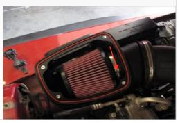
15. Install the other end of the Air Tube (H) onto the throttle body. Make sure that the coupler is seated properly on the throttle body. Tighten down the #44 Hose Clamp (J). Note: If equipped install the IAT sensor into the Grommet (R). Seat the sensor into the grommet until the O-ring is not visible and reconnect the wiring harness before installing the air tube onto the throttle body.
