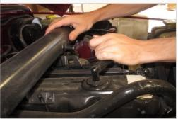
5. Remove three nuts securing the stock air box located under the passenger side wheel
