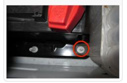
11. Unsnap the plastic clip holding the coolant reservoir to the AC line using a flat blade screwdriver. Then remove the other screw mounting coolant reservoir.
