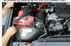
7. Loosen the hose clamp connecting the intake tube to the air box lid. Then remove the intake tube from the truck.
