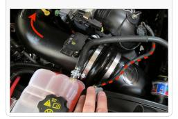
$23.\,$  Make any adjustments to Tube #2 (K) and Tube #1 (D) if necessary, when satisfied with the positioning, tighten all hose clamps. Do not over tighten. Reposition the Filter (E), if necessary, as stated in Step 20, making sure the filter is not rubbing against the Air Box (A), or touching anything and tighten the filter Hose Clamp (F).
