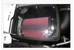
27. Reconnect both batteries and inspect your installation. Make sure the kit is properly positioned and all fasteners are secure. Affix the ID/CARB sticker near the intake kit. For 2015-2016 Models Only. Reinstall and bolt down both the upper & lower crossbars and side hood seal. Also re-insert the push pins on the front plastic
