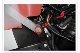
12. Carefully remove the MAF sensor from the stock air box lid and install the MAF sensor onto the Intake Tube #2 (K) with the supplied #8-32 Screws (O) and Plastic Spacers (N). Do not over tighten.
