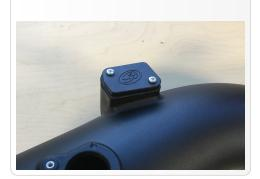
14. For 2013-2016 Models Only. Carefully remove the humidity sensor from the stock air box lid. Install the Gasket (P), the MAF Mount (Q), and humidity sensor onto Intake Tube #2 (K) with the supplied M4 Screws (S).
