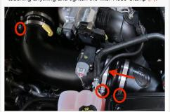
24. Reconnect the MAF sensor wiring harness. Reconnect the Humidity sensor wiring harness if applicable.
