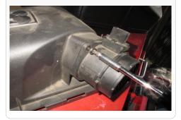
**20.** Install the factory MAF into the MAF Adapter in the S&B air box. This is designed to be a tight fit and may take some effort, carefully align the MAF Sensor to the Adapter.
