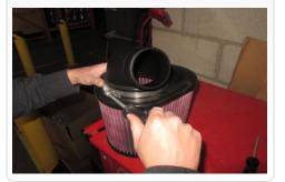
$28. \ \text{Install the S\&B air box, make sure the} \\$
