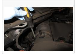
4. Use a 5/16" nut driver to loosen the hose
