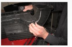
**16.** Push both grommets into part (K) Mounting
