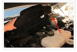
5. Pull the tube off the MAF and pull away.
