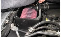
35. Install the Lid (N) onto the S&B air box using the provided hardware (P&Q) and the install is complete. Please make sure all hose clamps and hardware are tightened.
