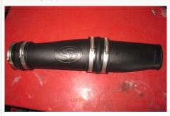
$\begin{array}{l} \textbf{26. Install the Hose Clamp (H) onto the MAF} \\ \textbf{Adapter (B)}. \end{array}$
