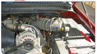
Remove the battery bolt and wedge then remove the battery from the vehicle.
