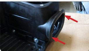
Install the Tube Seal (E) onto the Air Box (O).
