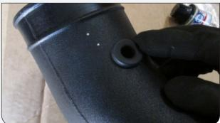
Install the Intake Tube (F) through the Tube Seal (E) from inside the Air Box (0). Pull out the intake tube until it reaches the stop bead.
