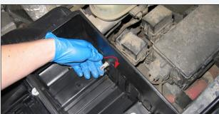
From the inside of the stock air box, turn the air temperature sensor a 1/4 turn to release it from the air box. Caution: Be careful not to damage the sensor.
