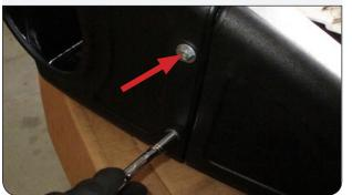
Install the Grommet (N) into the side of the Air Box (0).
