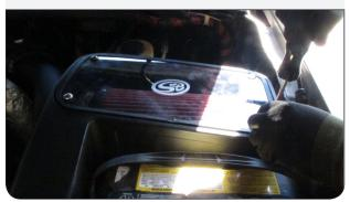
IF EQUIPPED: reconnect the electronic restriction gauge and push it into the grommet on the intake tube. Press firmly to ensure a air tight seal.
