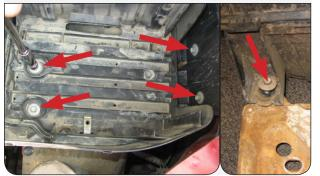
Remove the air box and tray from the vehicle. NOTE: Early 99' model stock air boxes have 2 bolts at the inner fender that need to be removed prior to the removal of the air box.
