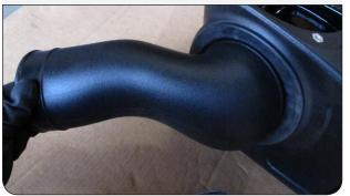
19 Slide the coupler with both hose clamps onto and over the intake tube. Push the coupler past both stop beads leaving the end of the tube exposed.
