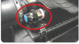
Unfasten and remove the stock air box lid and intake tube assembly from vehicle.
