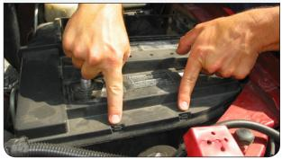
IF EQUIPPED: Disconnect the stock electronic restriction gauge electrical connector then read Step #16 and plan accordingly.
