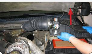
Remove the four bolts from the stock battery tray from the bottom and side. NOTE: Early 99' models have a separate bracket with a additional bolt. Remove this bolt as well, then remove the tray from the vehicle.
