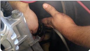
2 Use a paper or plastic funnel to refill your power steering fluid if needed. Reinstall the power steering reservoir cap.
