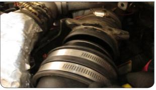
Install the Air Filter (M) onto the Intake Tube (F) and tighten the hose clamp. Make sure the filter flange is properly aligned with the stop bead before tightening completely. The filter and tube may need to be adjusted to fit straight with the box.
