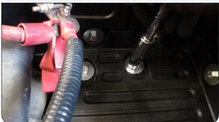
Install the provided M8 Bolts (U) and Washers (Q) to secure the Battery Tray (S) to the fender.
