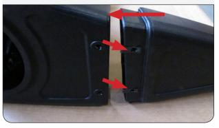
Secure the Battery Tray (S) to the Snorkel (A) and Air Box (O) with the 5/16"-18 Bolts (T), Washers (Q) and Lock Nuts (P). Do not over tighten.
