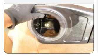
IF EQUIPPED: To reinstall the electronic restriction gauge drill a 3/4" hole in the Intake Tube (F) at the drill point and insert the Grommet (AB).
