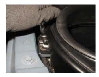
Install the Hump Coupler (Q) into the throttle body and tighten down the #52 Hose Clamp (P).
