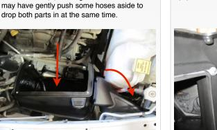
15. Insert the Air Inlet Tube (S) onto the Air Box (M) and secure using the supplied 1/4"-20x3/4" Screws (V), 1/4" Lock Washers (U) and 1/4" Flat Washers (W).
