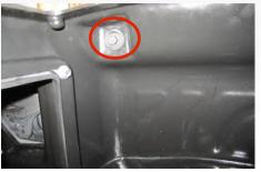
16. Reinstall the wheel liner using 6 of the OE screws. Reinstall wiring harness connector into wheel liner that was removed in Step #8.
