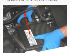
8. Loosen the hose clamp on the OE air box and remove the MAF sensor.
