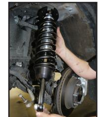
**8**. Connect the shock to the lower control arm: The lower shock mount has (1) long and (1) short spacer [Torque to factory spec]. Make sure the long spacer is toward the front of the vehicle as this will position the shock further toward the rear of the control arm to ensure adequate sway bar clearance. Install the factory lower shock bolt.
