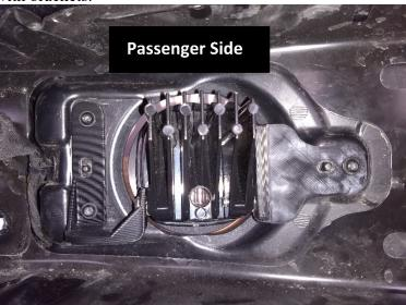
Step 6: With the two connectors included in the kit plug one side into the vehicle's harness and the other side into the Squadron's power cord. This will allow operation of the lights with the factory switch.
