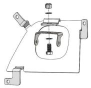
2. This kit places each Squadron light upside down inside the fog pocket. Using the 2.5mm Allen wrench, remove the four bezel bolts on the face of the light. Remove and spin the bezel and lense 180 degrees, then reinstall. Assemble the light onto the bracket with the rest of the hardware in the parts bag (see exploded view below). Tighten lightly for adjustment later. Repeat steps 1 and 2 for the opposite side light and bracket assembly.
