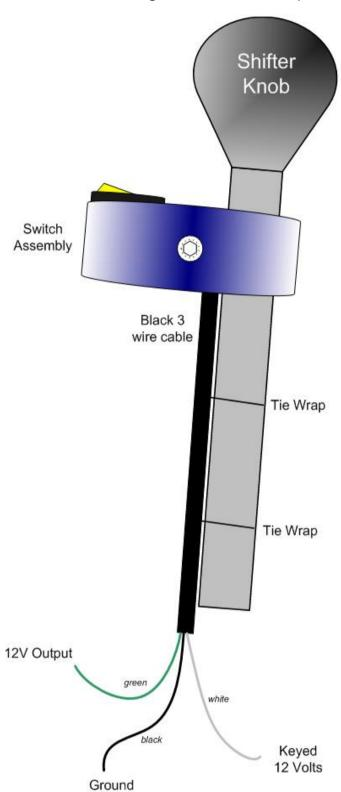
Posi-Tap connector to it (green for 10/12ga and black for 14/16ga wire). Connect the white wire of the rocker switch assembly to this Posi-Tap.
