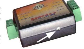
With the throttle at idle, start the engine and turn on brake switch. Then, using a small flat bladed screwdriver, turn the small adjusting screw in the DFIV Module counterclockwise or clockwise until the test light JUST turns on.
