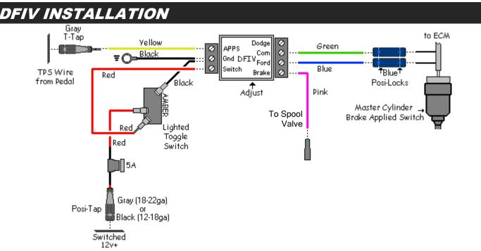
**CAUTION:** Before installing any wiring modifications or equipment ensure to disconnect the battery Ground (Negative) terminals on all the vehicle batteries as damage to the vehicle's ECU and/or installed components may result.
