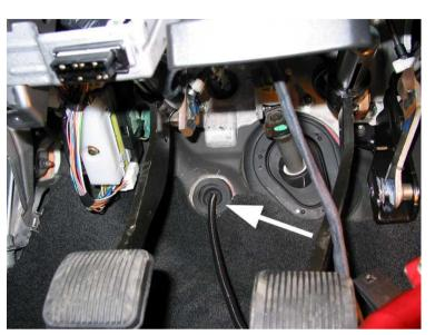
Open the loom and locate the Light Blue w/Black wire and install a supplied Posi-Tap<sup>™</sup> to it.
