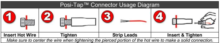
The ground terminals of the vehicle's batteries should be disconnected before performing any piercing/posi-tapping onto any ECM/PCM wire.
