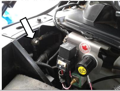
Connect the main power feed to the passenger side positive battery terminal clamp. This is the red wire with a ring terminal installed on the end.
