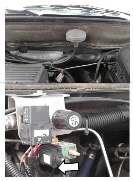
Connect the main ground connection to the body ground on the passenger side of the engine bay near the regulator assembly.
