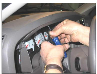
Note: Placing the transmission all the way into 1<sup>st</sup>/low gear and ensuring the tilt steering is all the way down will allow for easy removal.
