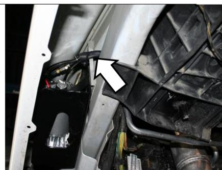
Secure the compressor in place by reinstalling the hood hinge bolt through the compressor bracket. Then install the nut and bolt to hold the front of the bracket.
