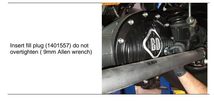
Some differentials may require special additives, please check your owner's manual before filling. Drive at least 50Kms (31 miles) re-torque bolts to specification ensure there are no leaks. Installation is complete.
