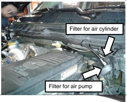
The preferred method of mounting the compressor air filter is just below the hood using a factory mounting location.
