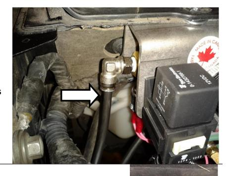
The other line from the compressor is the air suction line. This line is 1/4" diameter and comes with a preinstalled threaded adapter. Install the threaded filter supplied with the air pump into this fitting.
