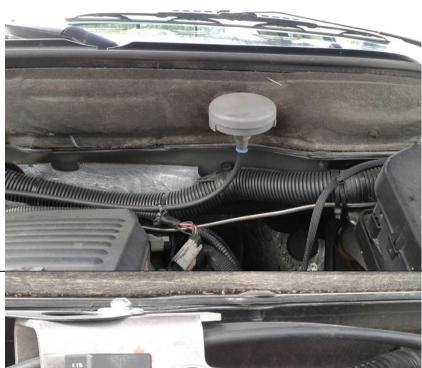
Locate the 1/8" tube from in the air tubing assembly that leads to the brake valve. This will be installed in the output from the air regulator assembly on the bottom of the solenoid.
