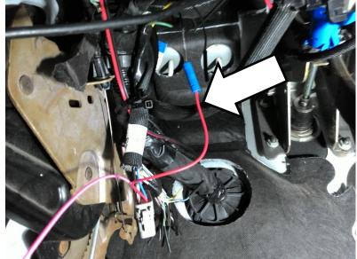
Fish the pink wire from the BD controller harness thru the firewall into the engine bay.
