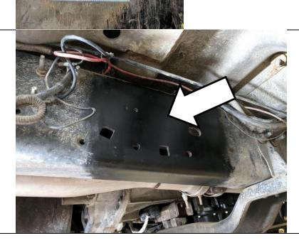
Position the two U bolts (MC-3060T54) on the frame, ensuring they are not pinching any wiring or tubes.
