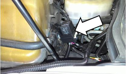
The ground wire (black wire with ring terminal) from the kit is installed with the body ground strap. Reinstall the bolt removed in the preceding steps.
