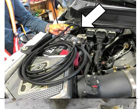
Route it alongside the pump air lines installed earlier and zip tie in place.
