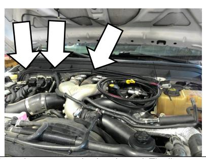
Depending on the routing of the airlines, they may need to be trimmed. The lines are supplied long to account for various line routings. Cut the tubing square and ensure the end is round so it will seal when installed.
