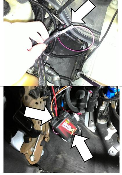
Apply the included exhaust brake decal to the AUX switch used to identify it as the exhaust brake switch.
