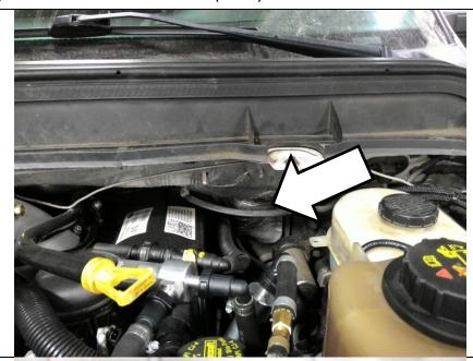
Remove the ground strap bolt on the top of the firewall.
