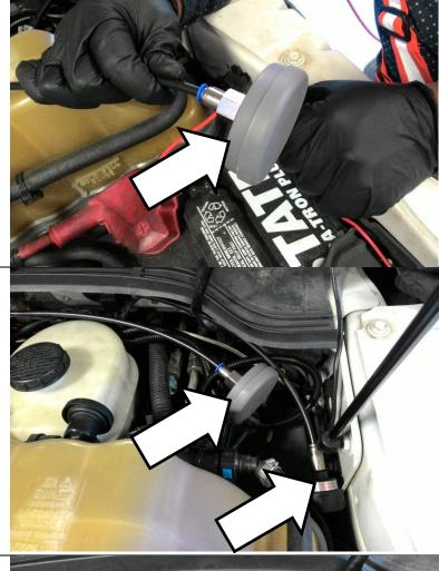
Position this line with the air filter and the other vent line in the corner of the engine bay, away from significant sources of heat or moisture.
