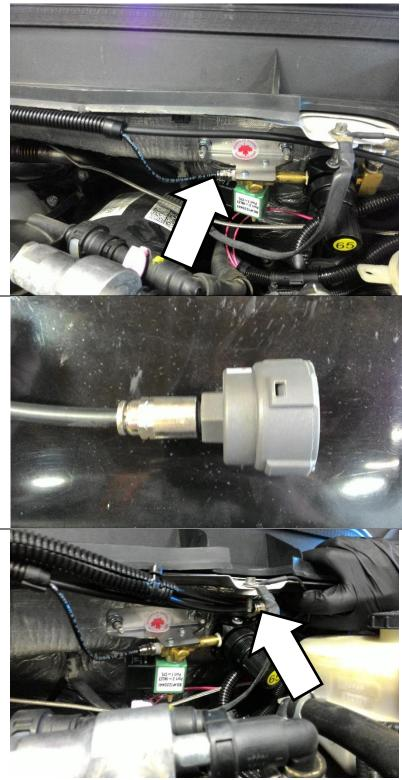
The other line from the air compressor is the suction line, this has the push on fitting to NPT adapter. Thread the supplied "pancake" filter into this fitting hand tight. This is the filter that came with the air compressor.
