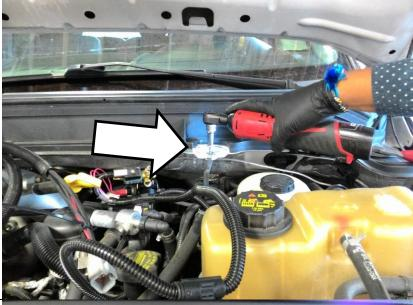
Position the regulator assembly (1220146) over the two M6 studs and install using the supplied M6 washers and nuts. Torque to 50 in-lbs.
